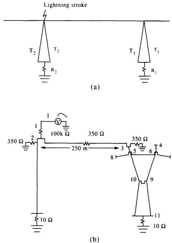
Fig. 2. Lightning stroke at tower  $T_2$ . System configuration: (a) schematic diagram; (b) system layout.
