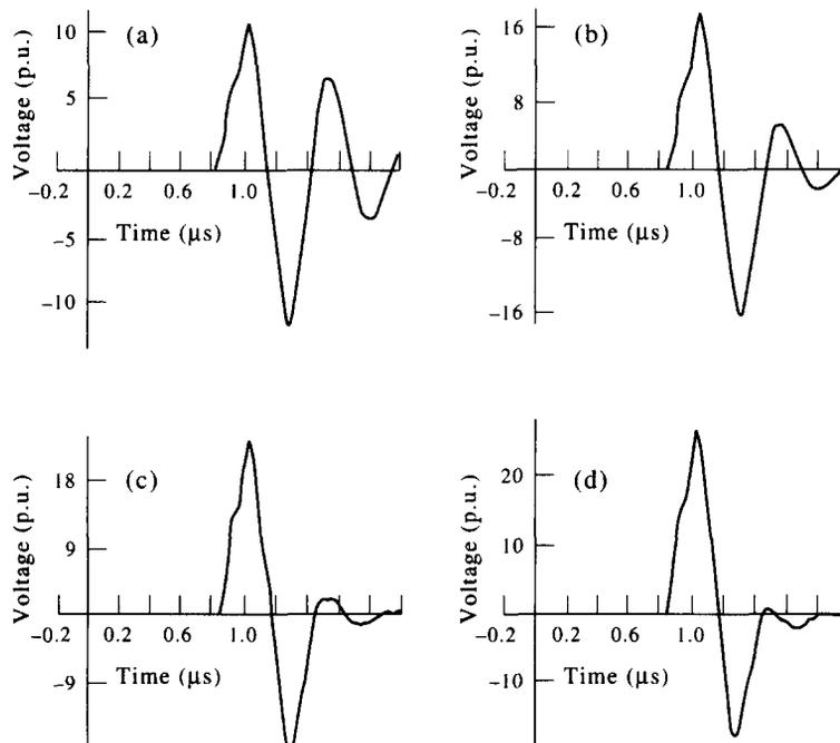
Fig. 7. Tower ( $T_1$ ) top potential ( $V_5$ ) for different tower surge impedance  $Z_1$  for a stroke at tower  $T_2$ : (a)  $Z_1 = 100 \Omega$ ; (b)  $Z_1 = 200 \Omega$ ; (c)  $Z_1 = 300 \Omega$ ; (d)  $Z_1 = 400 \Omega$ .
