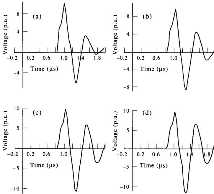
Fig. 5. Tower ( $T_1$ ) top potential ( $V_5$ ) for a 320 kA, 1.2/50  $\mu\text{s}$  stroke at tower  $T_2$ : (a)  $R_1 = R_2 = 10 \Omega$ ; (b)  $R_1 = 5 \Omega$ ,  $R_2 = 10 \Omega$ ; (c)  $R_1 = 1 \Omega$ ,  $R_2 = 10 \Omega$ ; (d)  $R_1 = 1 \Omega$ ,  $R_2 = 5 \Omega$ .
