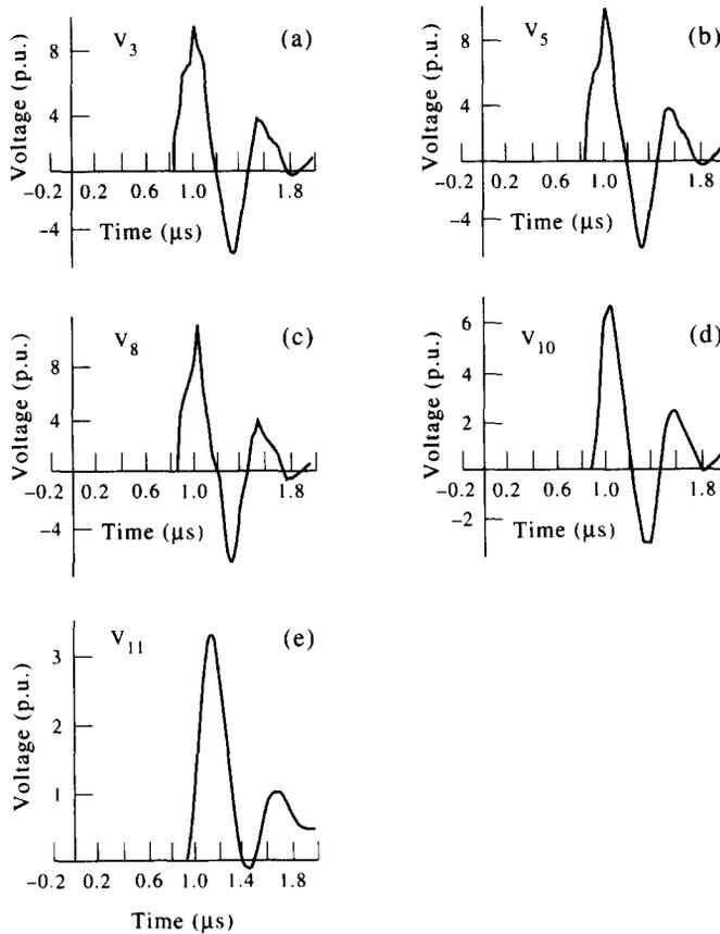
Fig. 4. Voltage at different points of the tower T<sub>1</sub> for a 320 kA, 1.2/50 μs stroke at tower T<sub>2</sub>.
