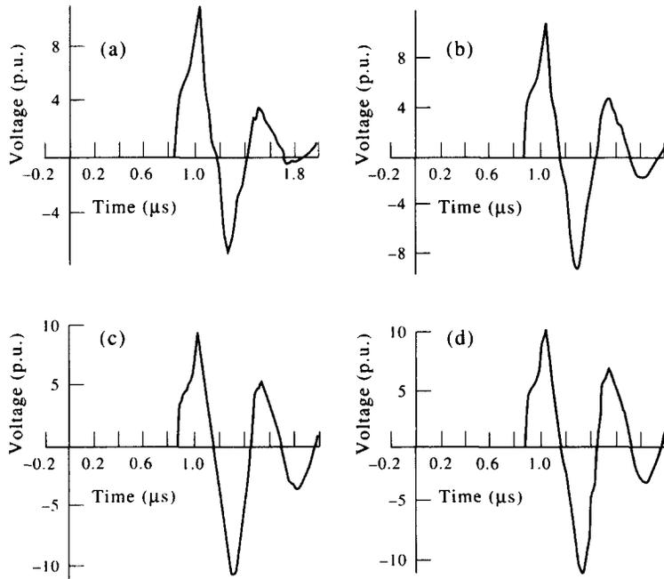
Fig. 6. Voltage at tower ( $T_1$ ) crossarm ( $V_8$ ) for a 320 kA, 1.2/50  $\mu\text{s}$  stroke at tower  $T_2$ : (a)  $R_1 = R_2 = 10 \Omega$ ; (b)  $R_1 = 5 \Omega$ ; (c)  $R_1 = 1 \Omega$ ,  $R_2 = 10 \Omega$ ; (d)  $R_1 = 1 \Omega$ ,  $R_2 = 5 \Omega$ .
